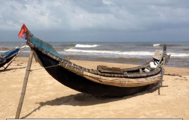
Upon closer inspection I noticed that these surf boats were crafted from woven bamboo. Necessity being the mother of invention, they were constructed from split bamboo that had been woven like a basket to form the hull, and then waterproofed with black tar. NGNGALKE
